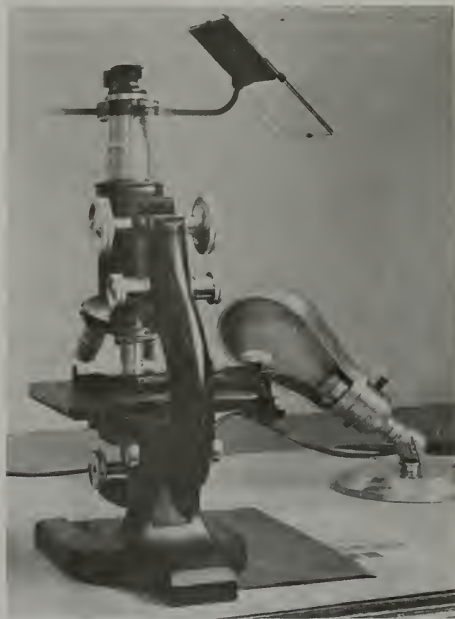
FIGURE 10. Microscope and modified Abbé-type camera lucida, showing position of black velvet used to block out one-half of the comparison field and one-half of the inclined mirror.
